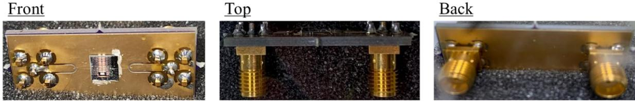
Figure S1. Example of a diced chip mounted on PCB and prepared for irradiation.
